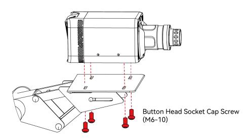
Method of mounting the base using regular rigs
