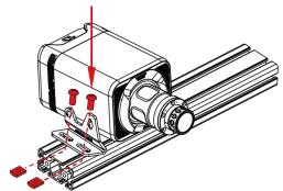
Roll in T-Nut with Ball Spring
