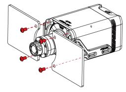
The pack includes Button Head Socket Cap Screw M8-14. If the length is not suitable, please select screws of the appropriate length based on your rig.
