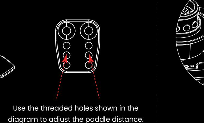
Use the threaded holes shown in the diagram to adjust the paddle distance.
