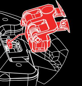
2.7 Plug the double-paddle assembly's cable into the connector on the steering wheel.
