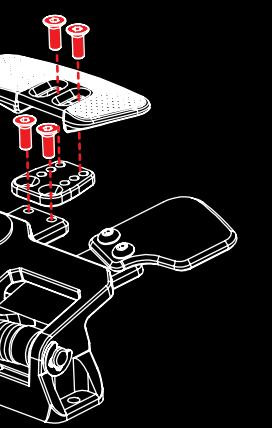
2.5 For metal paddles, use countersunk screws M3-6 to secure the paddle.
