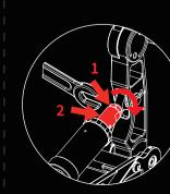
1. Loosen the jam nut on the back of the Brake, then spin the silver rod clockwise until completely loosened
