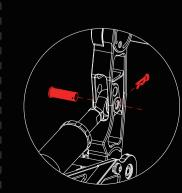
The Throttle resistance can be adjusted by switching the installation hole
