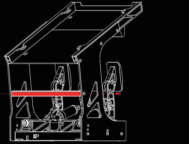
1. Loosen the two screws on both sides of the reinforcement bar with an Allen Key, remove the bar, then place the pedals in the inverted position
