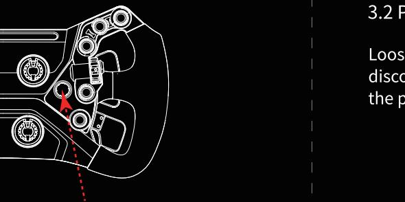
Push and hold both 7-way switches upwards for 5 seconds to enter Clutch Calibration mode, then press both clutches all the way down (then press any button) to complete the calibration (both clutches can be pressed simultaneously)
