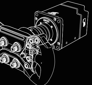
To pair the wheel to the wheelbase, attach the wheel and press the indicated buttons below to sync the frequency
