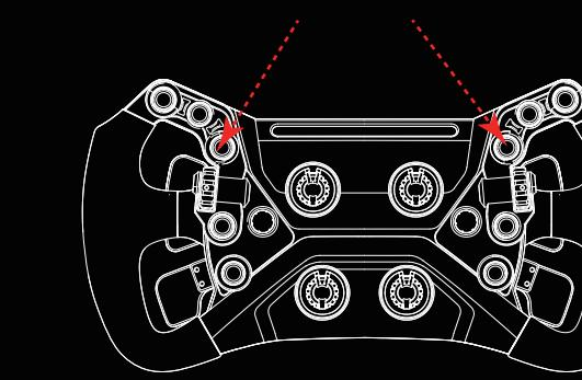
If there's no response when using the auto pairing mode, attach the included USB Type-C cable from the socket at the back of the wheel to the socket on the PC to manually sync the frequency (Please unplug the cable before driving in wireless mode )
