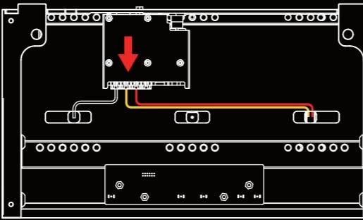
2.1 Remove the four screws on the brake module
