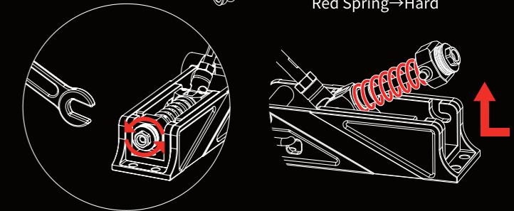
4.1 Rotate the rear adjustable screw to fine tune the spring force
