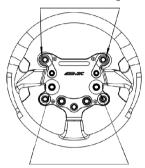
Press down the two buttons simultaneously for 5 seconds to enter Troubleshooting mode. When the mode is on, the lights keep switching to indicate a button or rotary is in working conditions or not.
