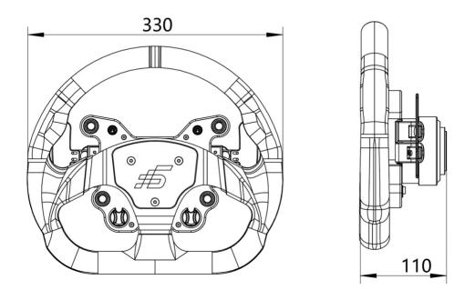
GT1D wheel diameter 330mm Plate mounting hole diameter 70mm PCD; 6xM5\*40 screws Quick Release mounting holes 70x6
