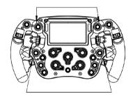
Press down the two buttons simultaneously for 5 seconds to enter Troubleshooting mode. When the mode is on, the lights keep switching to indicate a button or rotary is in working conditions or not.
