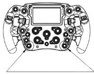
Press down the two buttons simultaneously for 5 seconds to reset to factory settings (only for the wheel)
