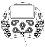
Push upwards the 7-way multi-position switch for 5 seconds to enter Clutch Calibration Mode
