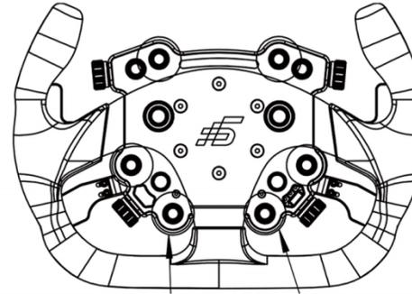
Press down the two buttons simultaneously for 5 seconds to reset to factory settings (only for the wheel)
