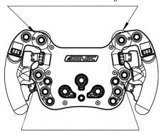
Press down the two buttons simultaneously for 5 seconds to enter Troubleshooting mode. When the mode is on, the lights keep switching to indicate a button or rotary is in working conditions or not.
