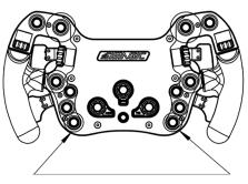
Press down the two buttons simultaneously for 5 seconds to reset to factory settings (only for the
