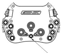
Push upwards the 7-way position switch for 5 seconds to enter Clutch Calibration Mode
